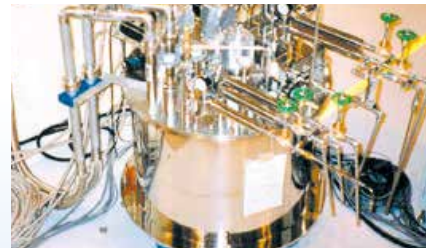
Circulation Unit & Vacuum Jacketed piping
